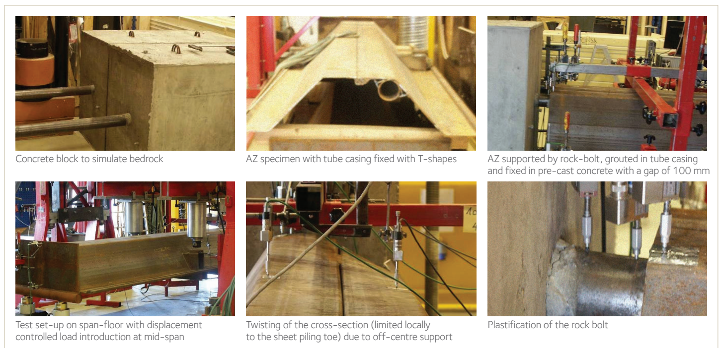
Pict. 5. Pictures of laboratory tests performed by the NGI
