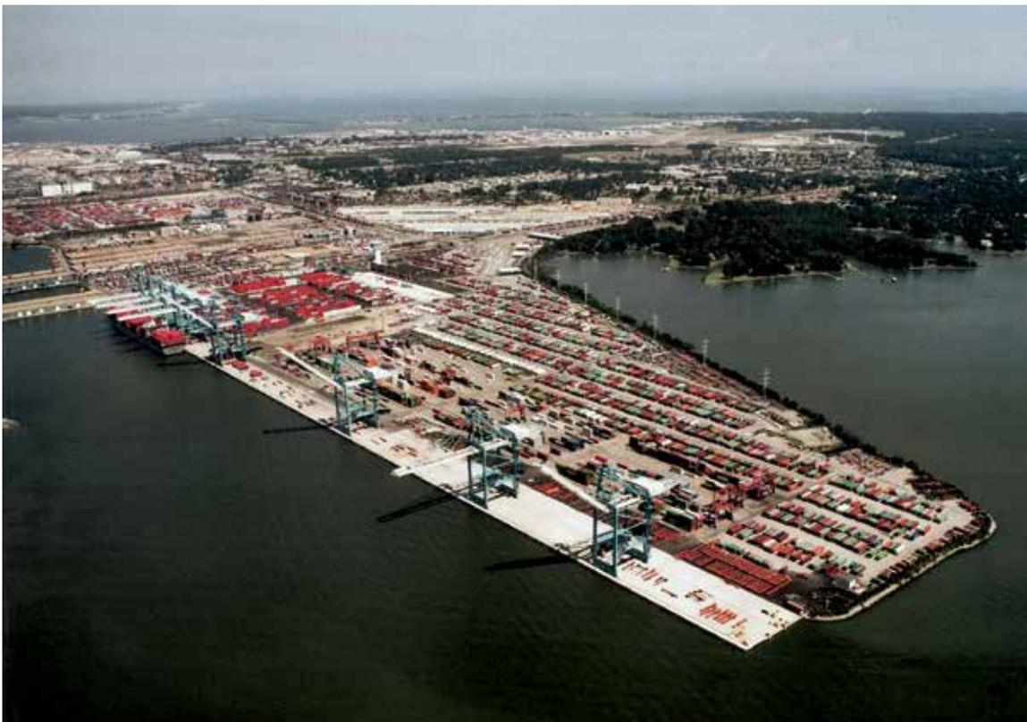
The NIT south wharf was renovated using two rows of steel sheet piles.
