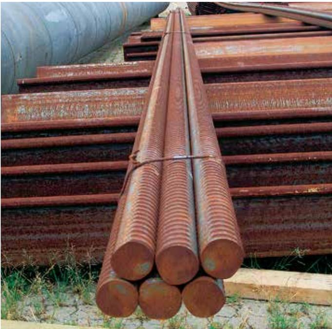
The tie rod consists of a 28 m steel bar, 56 or 63 mm in diameter.
