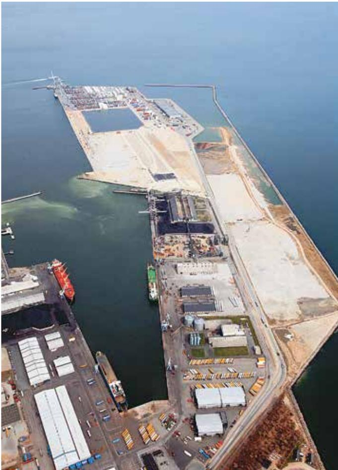
Some 3.5 Mm<sup>3</sup> of sand were placed behind the sheet pile wall to create the new CT East.
