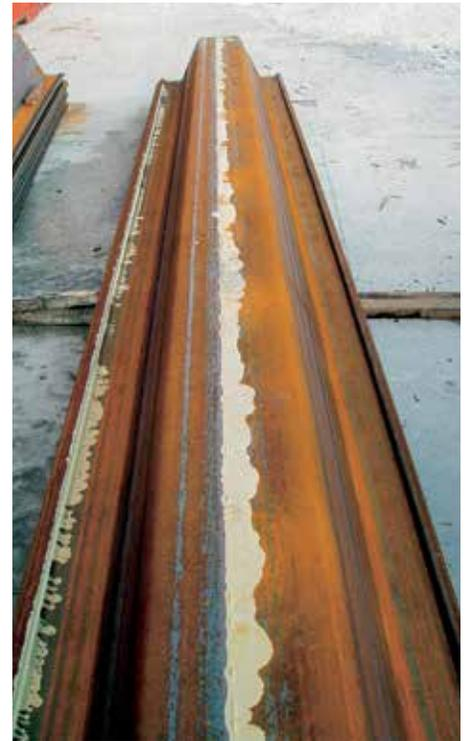
*A sealing system, the waterswelling Roxan system, was inserted into the piles interlocks.*
