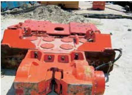
The driving gear consisted of a vibratory hammer...
