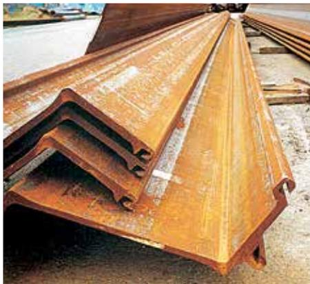
Several special piles and one PU pile were required to form the walls' corners and to attach the new quay wall to the existing structure. The following special piles were supplied by a subcontractor of ArcelorMittal and shipped to Taiwan together with the other sheet piles:
