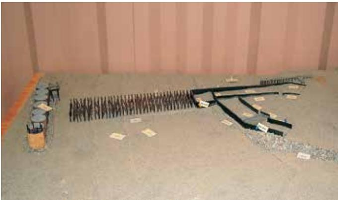
*The breakwater consists of sheet pile cells assembled with straight-web sections, whereas bending-moment-resisting sheet piles were used to build the terminal walls.*
