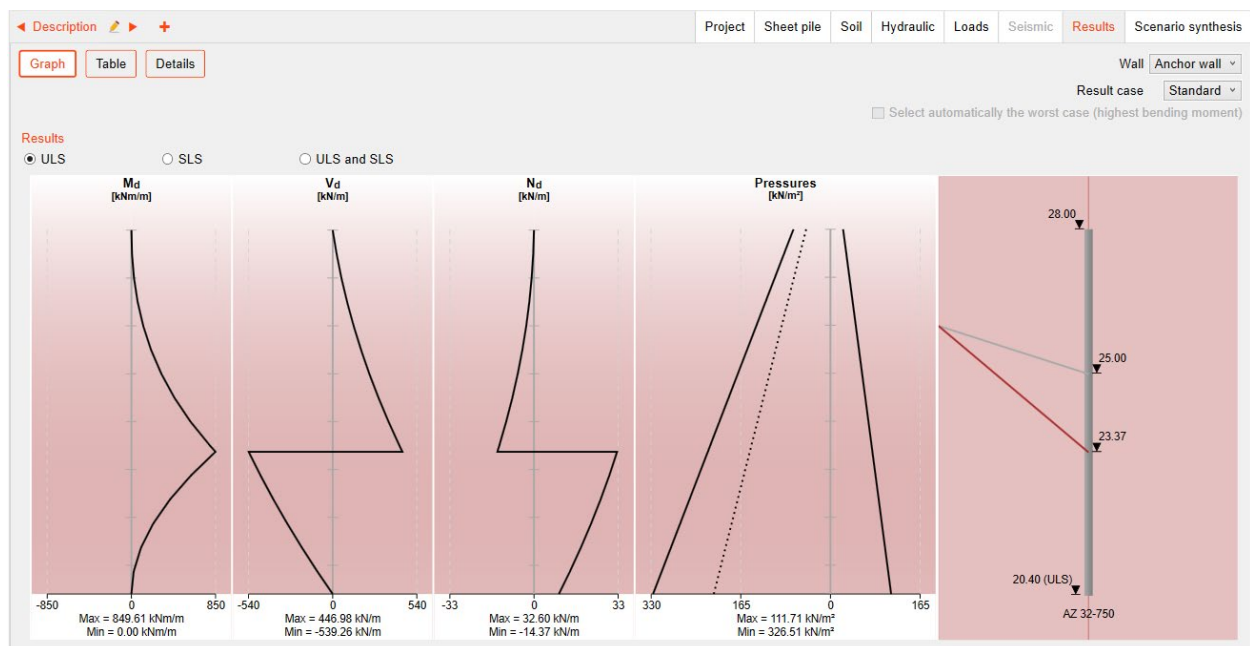
Figure 28. ULS results (graphs for anchor wall)
